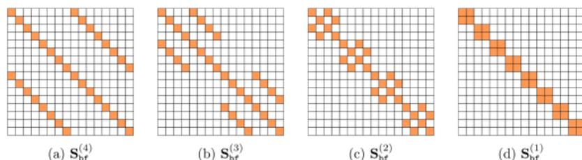
Figure: Butterfly structure:  $\text{supp}(\mathbf{X}^{(\ell)}) \subseteq \mathbf{S}_{br}^{(\ell)} := \mathbf{I}_{N/2^\ell} \otimes \begin{bmatrix} 1 & 1 \\ 1 & 1 \end{bmatrix} \otimes \mathbf{I}_{2^{\ell-1}}$ .
