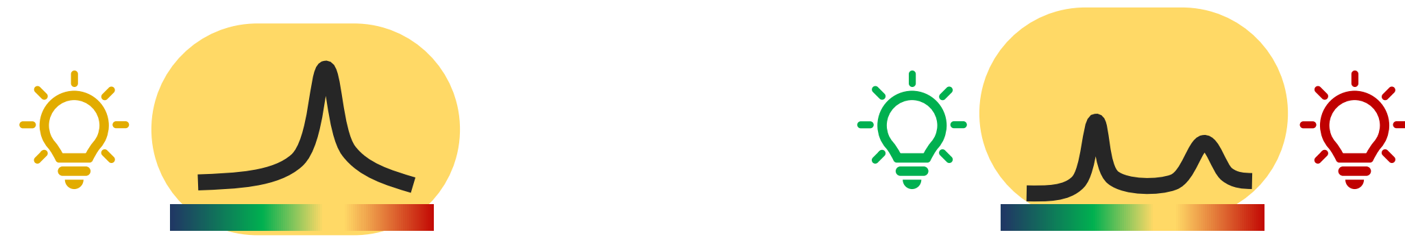
Fig. 1. Example of a metamer – (left) Monochromatic (590 nm) and (right) dichromatic (525 (green) and 625 (red) nm) light sources that are both yellow.
