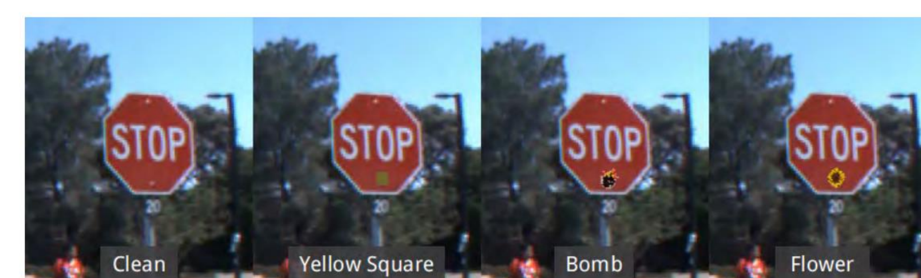
Fig. 2. A stop sign from the U.S. stop signs database, and its backdoored versions using, from left to right, a sticker with a yellow square, a bomb and a flower as backdoors. The backdoored images are mislabeled to speed limit sign. (This figure is from [1].)
