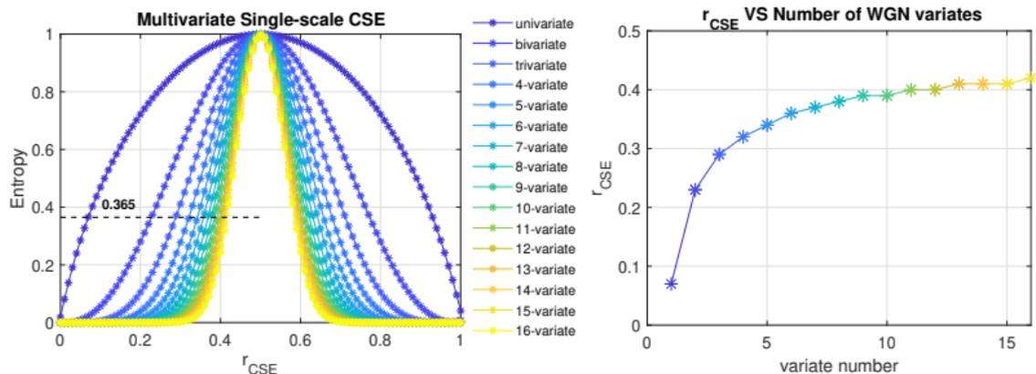
Figure 2: Behaviour of the Multivariate Single-scale CSE on the estimation of White Gaussian Noise (WGN), as a function of the tolerance,  $r$ .
