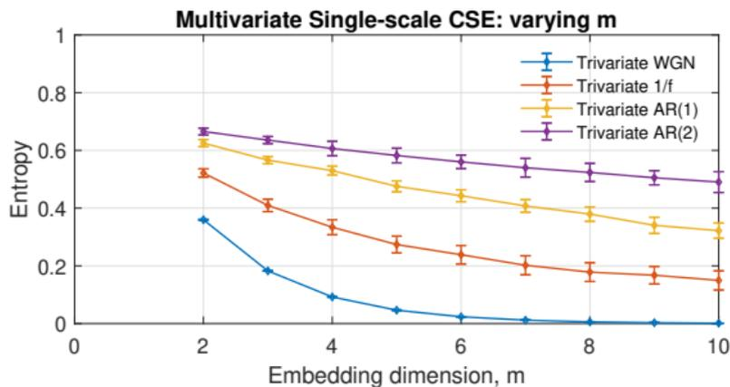
**Figure 3:** Multivariate Single-scale CSE as a function of the embedding dimension,  $m$ .
