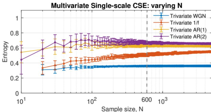
**Figure 4:** Multivariate Single-scale CSE as a function of the number of sample points,  $N$ , evaluated for the same four synthetic models. The default parameters are set as  $m = 2$ ,  $r = 0.287$ , and  $l = 1$ .
