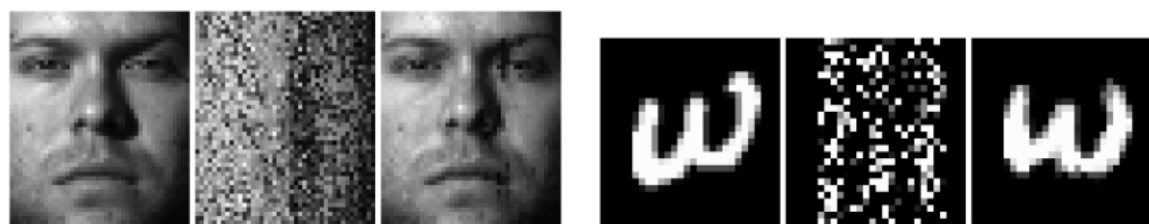
Left. Input image. Middle. Scrambled image. Right. Reconstruction by algorithm.
