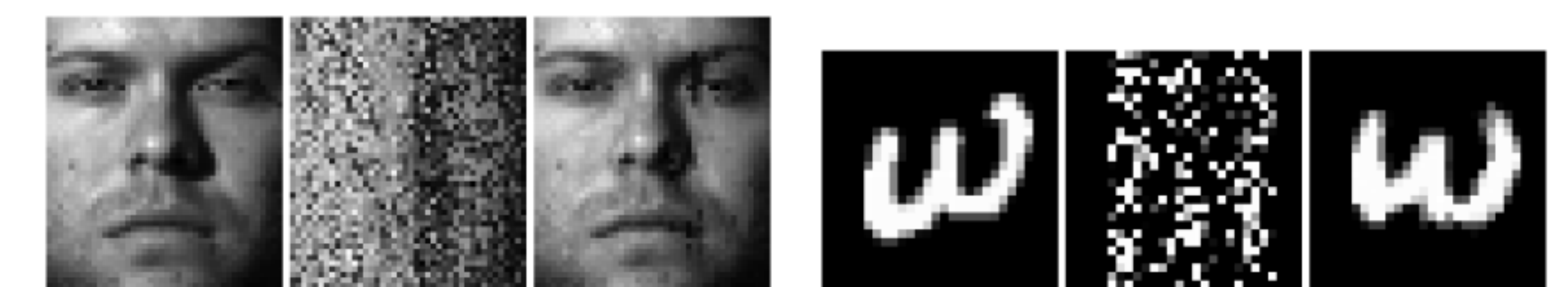
Left. Unscrambled input image \mathbf{y} from the YALE B and MNIST dataset. Middle. Scrambled input image \mathbf{P}\mathbf{y} . Right. PAM reconstruction \hat{\mathbf{y}} = \hat{\mathbf{P}}^\dagger \mathbf{P}\mathbf{y} .
