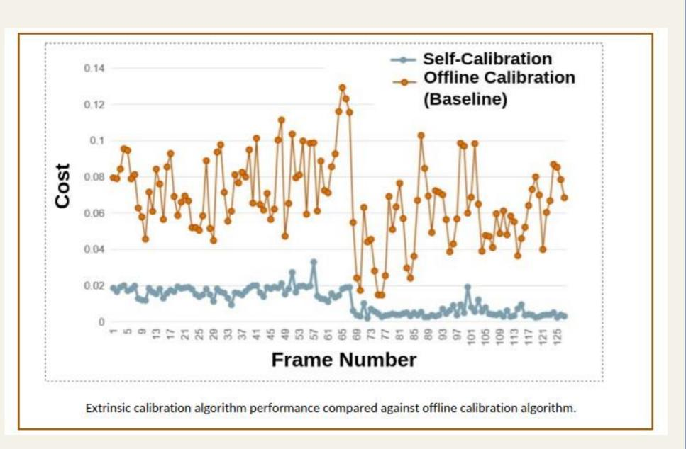
Alignment of detected lane boundaries in the camera with lane boundaries obtained from the map is used to assess the quality of camera calibration parameters. From the graph, it is evident that the self-calibration algorithm estimated extrinsic are more accurate than those obtained
