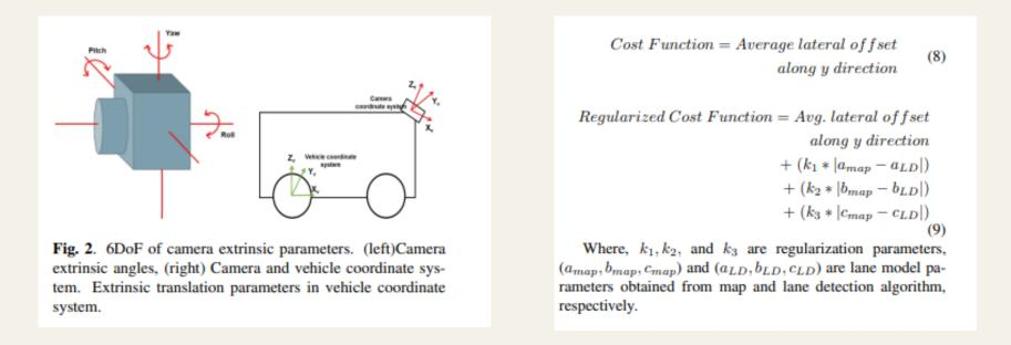
After this, the average cost is calculated for all samples. If this Average Cost is greater than the Convergence Threshold, the sample with minimum cost is selected, and new samples are generated around that minimum cost samples. Fig3 : Test Track [I275 Interstate Highway, Michigan, USA], Route Distance : 4miles approx.
