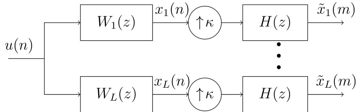
The oversampled control signal from woofer I is sent through the MDC encoder resulting in K descriptions.
