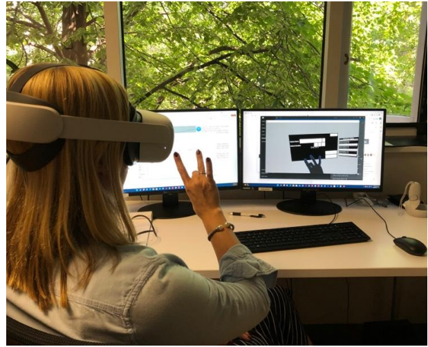
Figure 4. Original experimental setup. Participants can see the UI in VR environments, and their view is mirrored on the computer.
