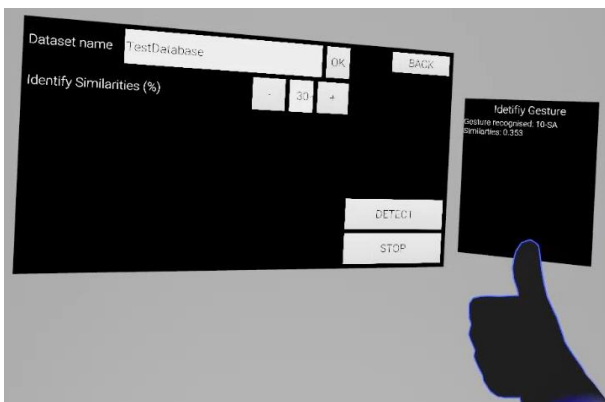
Figure 3. ASL number recognition UI. The detected gesture is shown in the right window with a confidence value.
