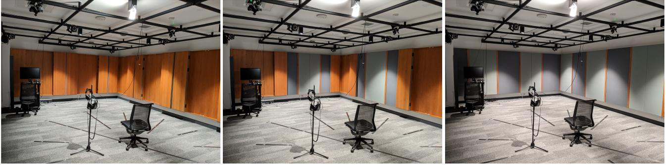
**Fig. 1.** Variable acoustics laboratory with three acoustic panel configurations: fully reflective (left), 50% absorptive (middle), fully absorptive (right).
