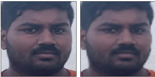
Fig. 3: An illustration of low-resolution augmentation is provided in this example. The initial image is presented as the original, while the subsequent image demonstrates the effect after applying the low-resolution augmentation technique.
