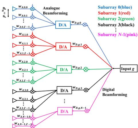
Figure 2: Localised subarray architecture.
