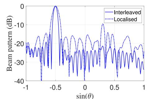
Figure 3: Resultant responses of the 0th beam generated by design (7).
