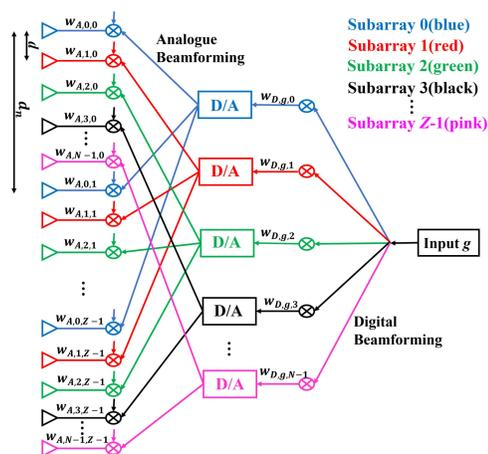
Figure 1: Interleaved subarray architecture.
