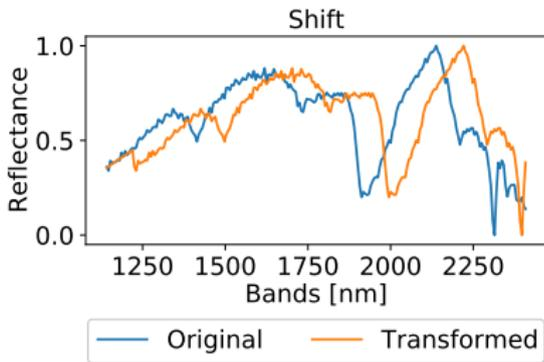
Figure: Spectral Shift Transformation.
