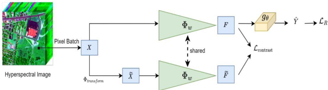
Figure: Architecture of the proposed method.
