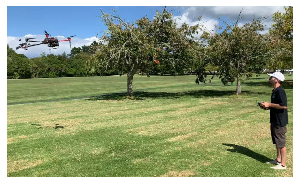
Fig. 6. Recording UAV in-flight rotor noise.
