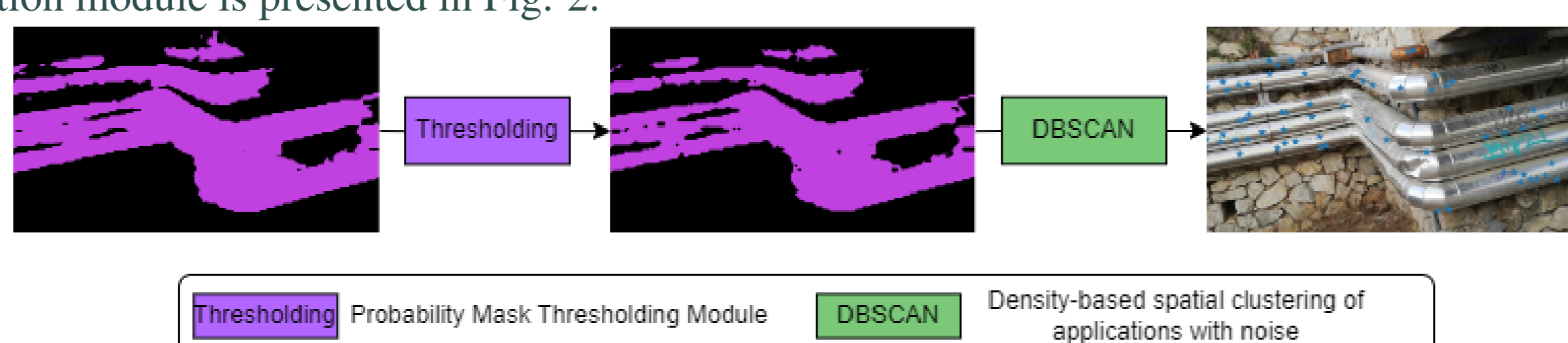
Figure 2: Point extractor Module extracts from a thresholded version of the CNN segmentation mask point that lay on the pipes. These points are used to prompt the the SAM in the later stages of the proposed system.
