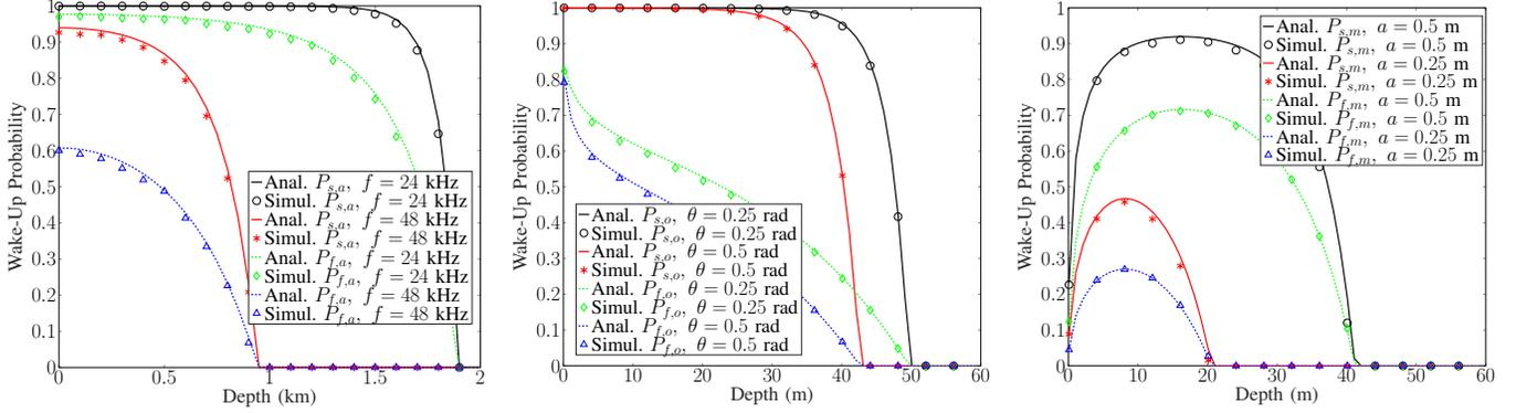
Fig. 3: Success and false probabilities for acoustic-based wake-up scheme. Fig. 4: Success and false probabilities for optical-based wake-up scheme. Fig. 5: Success and false probabilities for MI-based wake-up scheme.
