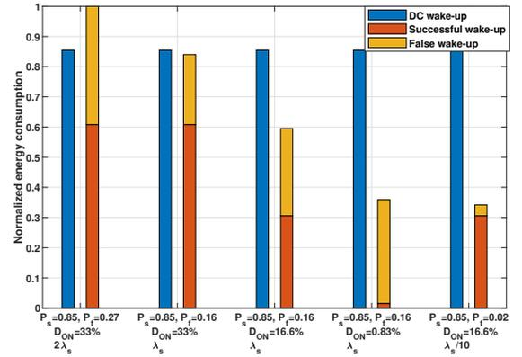
Fig. 6: Energy consumption of the proposed wake-up solution and the duty cycling technique under different settings.
