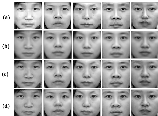
Fig. 2. Visual results of our SCFR-FSR method. (a) LR face images, (b) reconstructed initial HR face images, (c) final SR face images, and (d) original HR face images.
