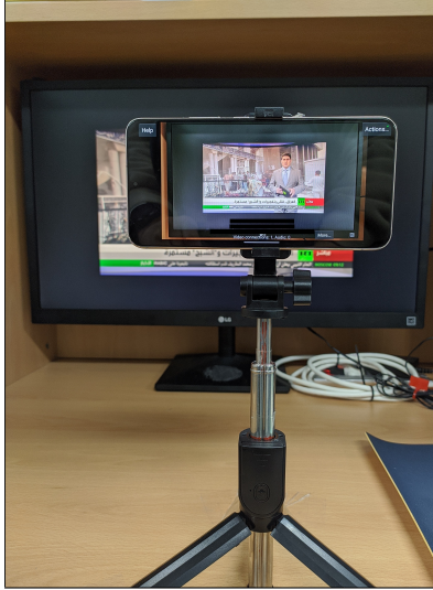
Fig. 2. The experimental setup involves the playback of videos sourced from FF++ and CelebDF on a computer screen. Subsequently, these videos are recorded using a smartphone camera. This method allows for the capture of the inherent Moiré pattern induced on the computer screen within the recorded video.
