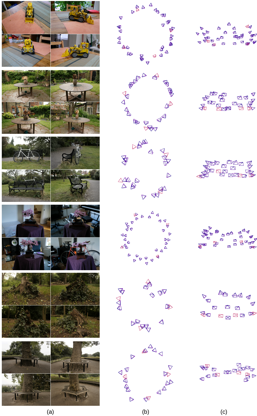
Fig. 2: Training images and camera distribution for selected scenes from the Mip-NeRF 360 dataset (kitchen, garden, bicycle, bonsai, stump, and treehill). (a) Training images; (b) top view of camera distribution with training cameras in red and test cameras in blue; (c) side view of camera distribution with training cameras in red and test cameras in blue.
