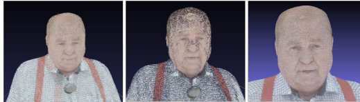
Fig. 2. The same underlying point cloud can have highly different quality characteristics depending on rendering parameters and the radius of interaction, especially in the NR setting. Point cloud taken from LS-PCQA and rendered in MeshLab. Best viewed zoomed in.
