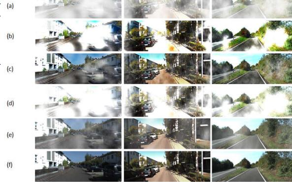
Fig. 8 Heavy fog exists in Road images: (a) Foggy images of residential, city and road; (b) He et al.'s result; (c) Meng et al.'s results; (d) Zhu et al.'s results; (e) Our results; (f) ground truth images.
