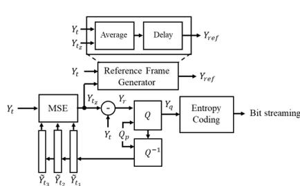
Figure 2. Proposed of compressed-domain inter-coding architecture.
