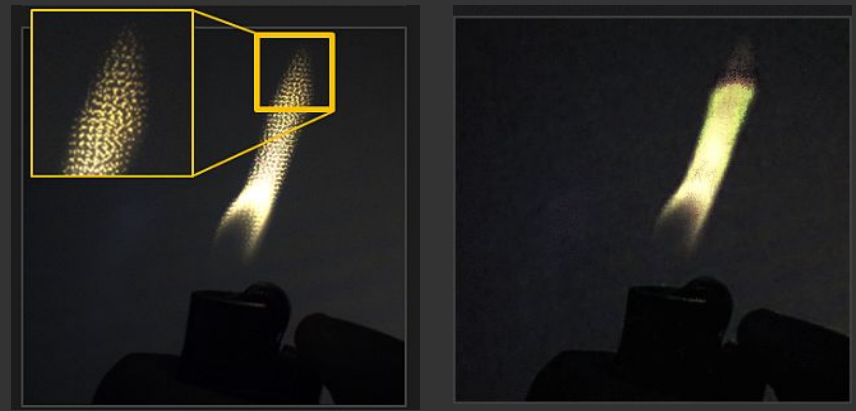
Video from single coded image (Hitomi et al '11)
