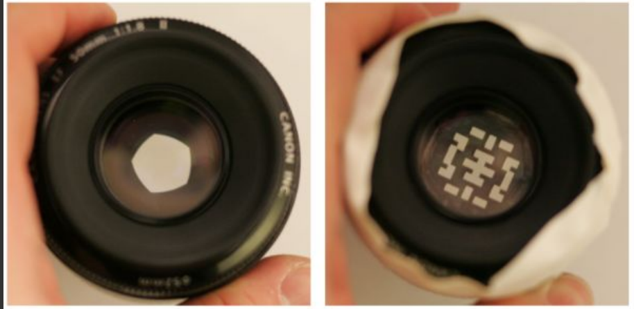
Coded Aperture for Defocus deblurring (Levin et al '06)
