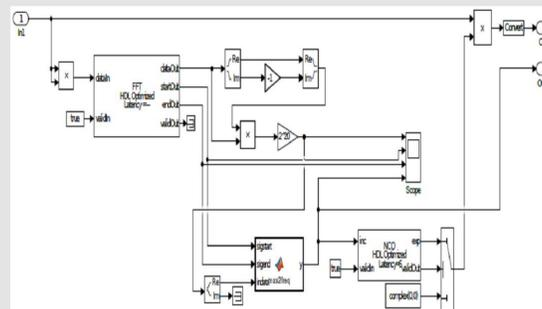
Fig. 2: HDL compatible frequency offset compensation block design
