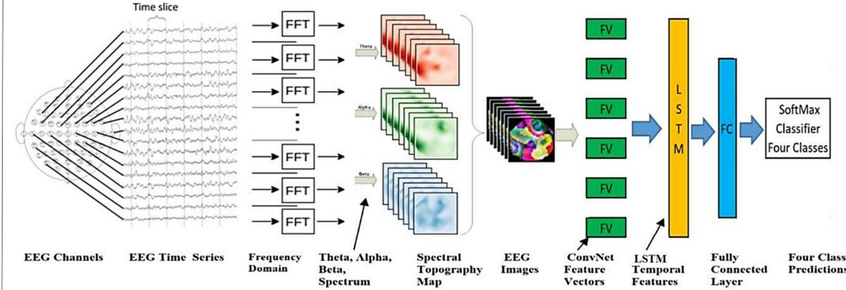
Framework overview: (i) EEG signals from multiple cortex locations (ii) FFT and topographical maps (iii) Spectral maps combined to form 3 channel images, (iv) CNN (ConvNet) FV and LSTM for representation learning (v) Softmax classification.
