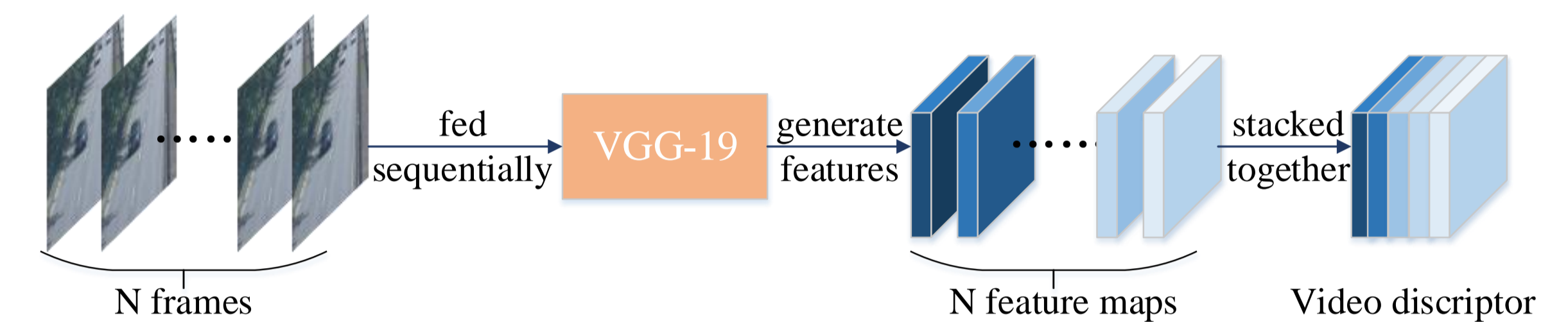
Figure 2. The architecture of the feature extraction network.
