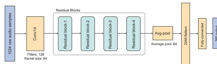
Figure 2. Network architecture of DeepFO.
