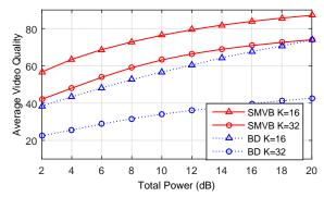
**Fig. 1.** Video quality of multi-user beamforming schemes with K users, N=4 cooperating base stations,  $N_u=4$  transmit and  $N_b=4$  receive antennas.
