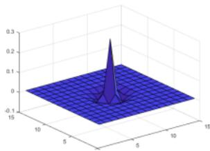
Example of center-surround filter using difference of two Gaussians.
