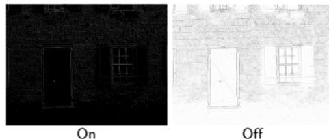
Example of the positive (on) and negative (off) response when using a center-surround filter.
