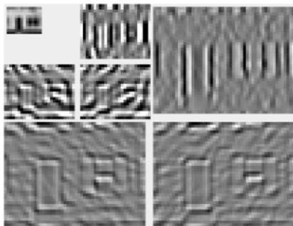
Output of a wavelet pyramid with 2 stages and 3 orientated wavelets
