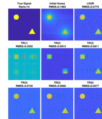
Figure 3. Reconstructed image of the simple geometric shape using unregularized TR with  $R = 1, \dots, 6$ , and LSQR.
