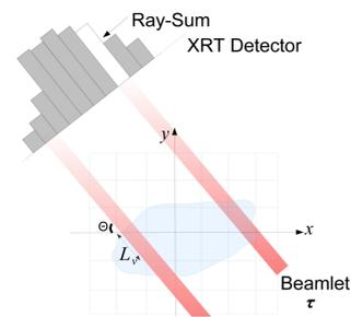
Figure 1. Discrete XRT projection geometry
