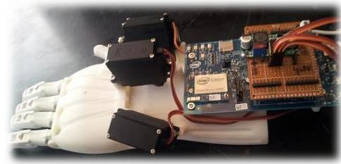
Figure 4: The constructed prosthetic hand.
