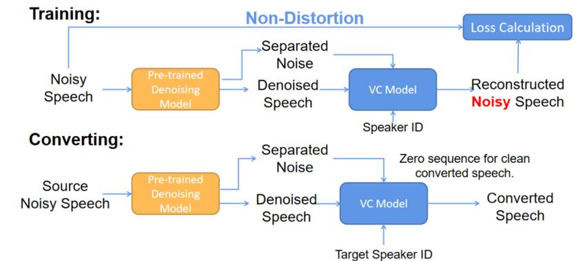
The modified VC model: noise-conditioned vector-quantized variational autoencoder (VQ-VAE)
