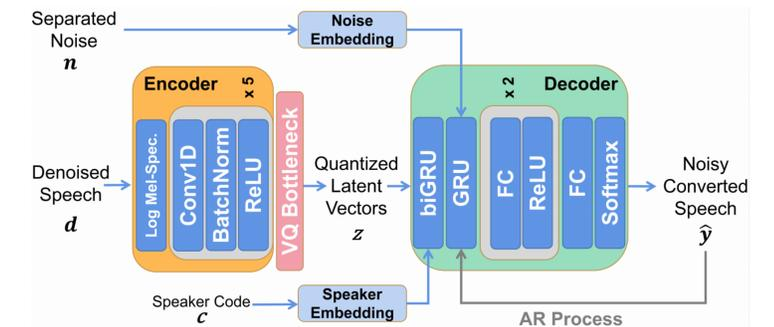
The decoder takes the noise signal as a condition to model the joint probability distribution of the noisy speech:
