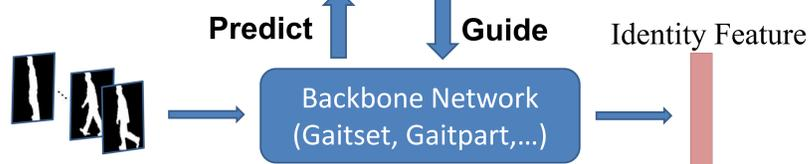
➤ In this paper, we proposed a **general framework for multi-view gait recognition** by explicit view angle embedding, based on which, two state-of-the-art gait recognition backbones, i.e. Gaitset and GaitGL are enhanced. Compared with the original ones, the enhanced ones, improve the performance. The effectiveness is well demonstrated by the experiments on CASIA-B and OUMVLP datasets.
