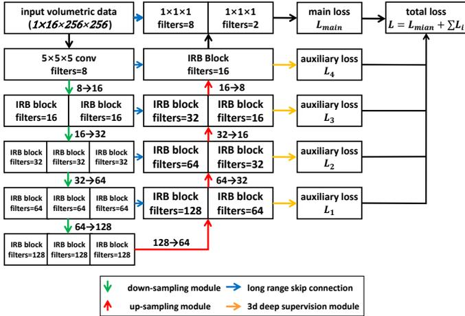
Fig. 1: The detailed structure of LV-Net.
