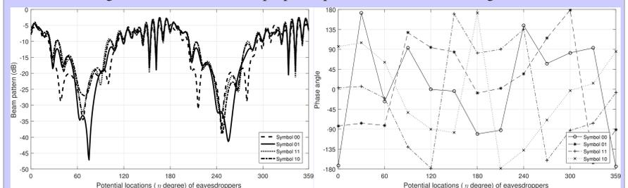
Figure 2: Resultant beam pattern based on the ULA design
