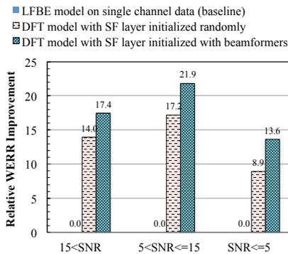
Fig. 6. Effect of initialization of the SF layer.
